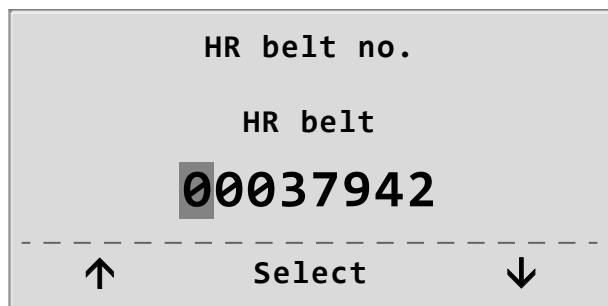
Figure 6–31: Setting the HR belt no. – screen 2
