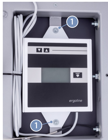
Figure 4-15: Control terminal under the couch surface
