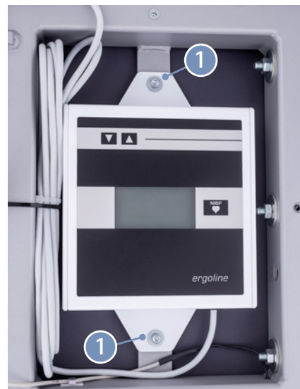
Figure 4-15: Control terminal under the couch surface
