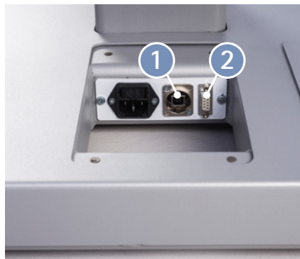
Figure 4 – 13: Connection for ECG recorder/PC ECG system
