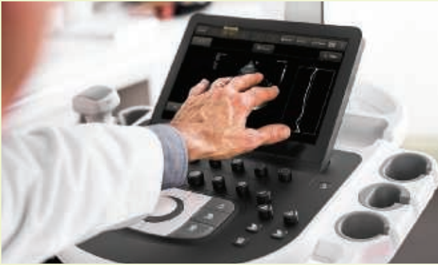
With image replication and TGCs on its tablet touchscreen, Affiniti 50 was designed to reduce reach and button pushes.
