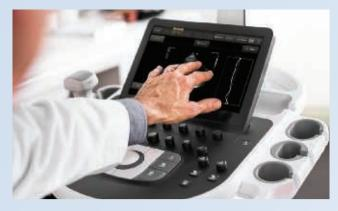
With image replication and TGCs on its tablet touchscreen, Affiniti 50 was designed to reduce reach and button pushes.
