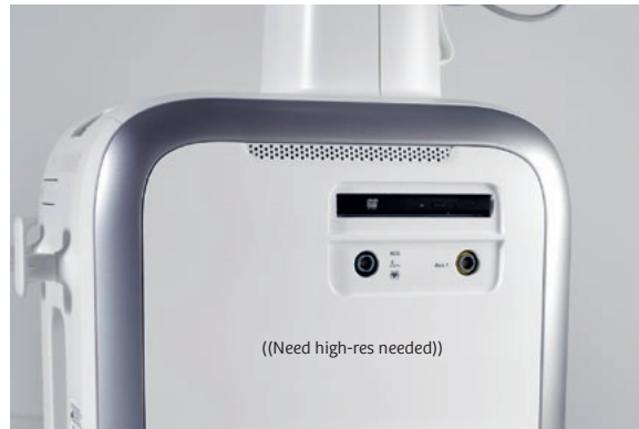
ECG cable connector, DVD writer and physio port.
